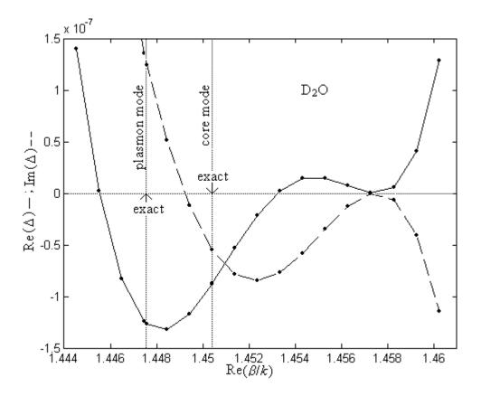
Fig. 2. The real (solid line) and imaginary (dashed line) parts of the determinant  $\Delta$  corresponding to the dispersion equation versus the real part of the effective index for  $HE_{11}$  core and plasmon modes near the loss matching point ( $\lambda = 0.61581 \mu$ m) when the analyte is heavy water for a fiber with four layers.
