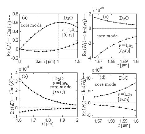
Fig. 4. The real and imaginary parts of the Bessel function J in the core layer (a), modified Bessel function K in the analytical layer (b) and Hankel functions  $H_1$  in (c) and  $H_2$  in (d) in the gold layer at the loss matching point ( $\lambda = 0.61576 \mu m$ ) of the core mode  $HE_{11}$  when the analyte is heavy water for a fiber with four layers.
