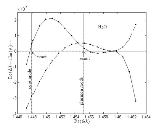
Fig. 3. The real (solid line) and imaginary (dashed line) parts of the determinant  $\Delta$  corresponding to the dispersion equation versus the real part of the effective index for  $HE_{11}$  core and plasmon modes near the loss matching point ( $\lambda = 0.5655 \mu$ m) when the analyte is distilled water for a fiber with three layers.
