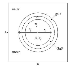
Fig.1. Cross section of an optical fiber with four layers made by SiO<sub>2</sub> core (radius  $r_1$ ) surrounded by a GaP layer (thickness  $r_2 - r_1$ ), a gold layer (thickness  $r_3 - r_2$  and by a water layer which can be considered infinite for the numerical model.
