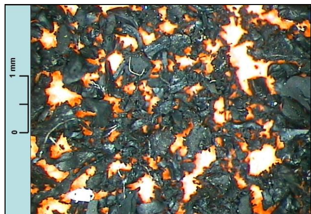
C 0.1-0.4 ("fine", ambient size reduction) Visible presence of metal and textile impurities
