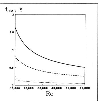
Figure 2. Dependence of the turbulent mixing time on the operating parameters.
