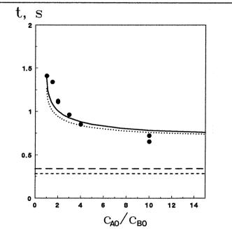
Figure 3. Comparison of the experimental results by Pohorecki and Baldyga (1983) [•] and the predictions of the three-stage micromixing model.
