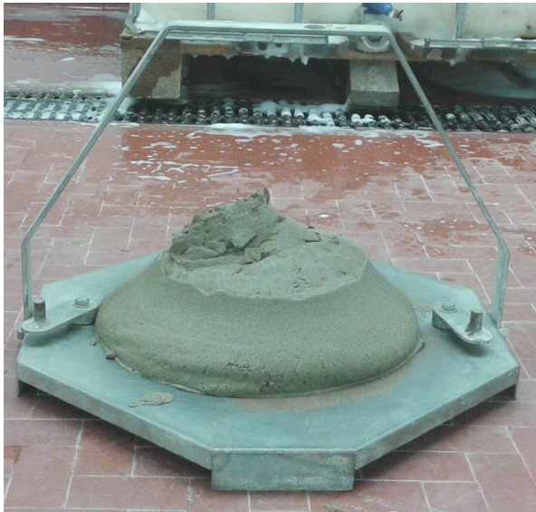
Figure 3.4: Optimal conditioning slump for Soil A
