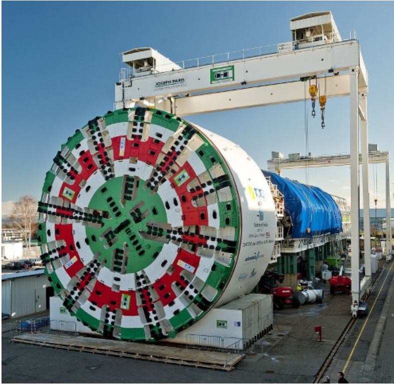
Figure 1.3: Martina EPB Sparvo, Italy. (from TOTO SpA web site). With a maximum excavation diameter of 15.61 m, weight 4500 t, maximum thrust force 400000 kN at 500 bar, installed power 16800 kW.
