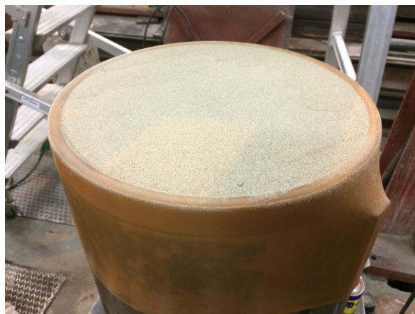
Figure 6.20: Levelled surface of the sample before the connection of the top cap with the membrane
