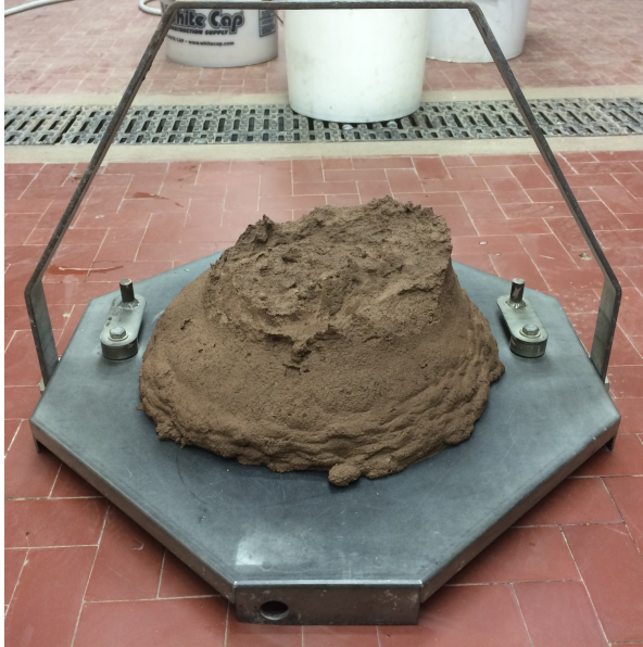
Figure 3.16: Optimal conditioning slump for Soil E
