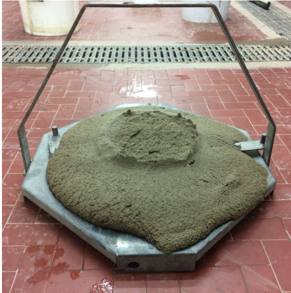
Figure 7.79: Slump test carried out on conditioned Soil A extracted from the test.
