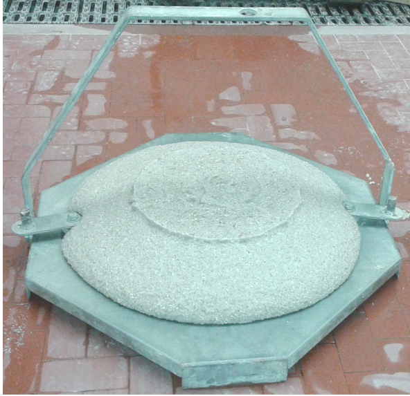
Figure 3.14: Optimal conditioning slump for Soil D
