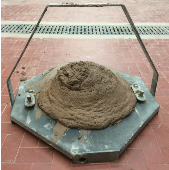
Figure 7.85: Slump test carried out on conditioned Soil E extracted from the test.
