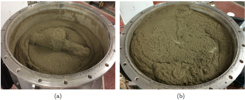
Figure 7.78: Conditioned material at the beginning of the test (a) and after the cycle increase/decrease of pressure at 500 kPa (b).
