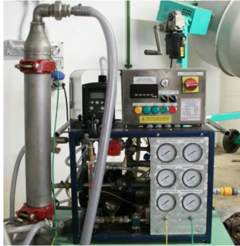
Figure 2.1: Lab scale foam generator at TUSC laboratory.
