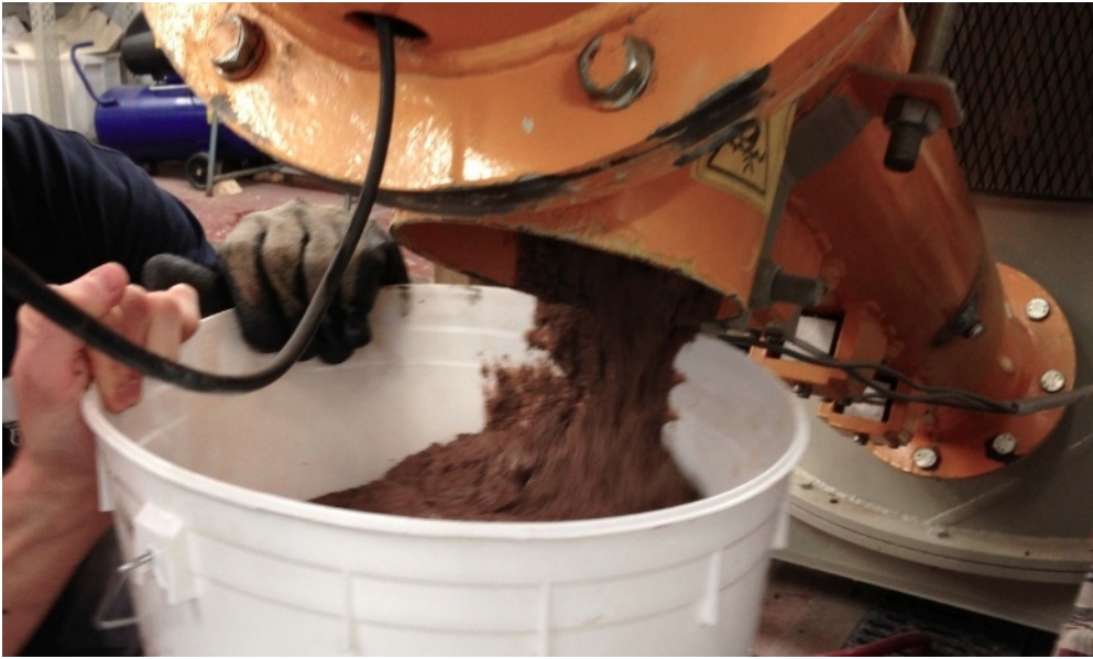
Figure 3.29: Flow of the material from the screw conveyor.
