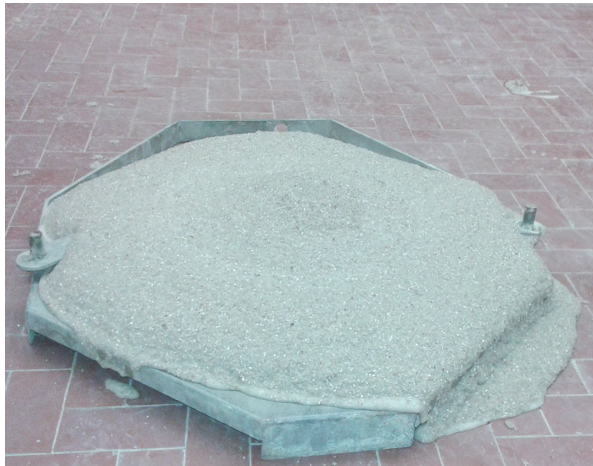
Figure 3.13: Slump for Soil D without adding fine material
