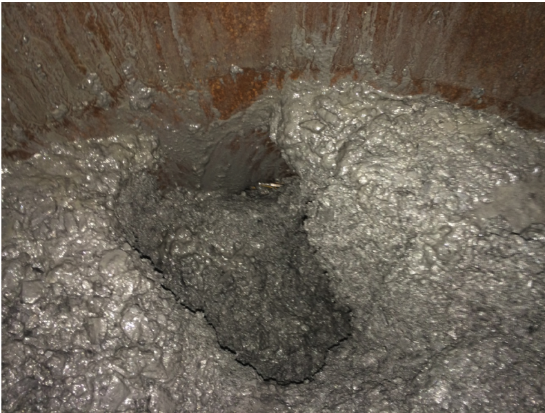
Figure 4.3: Creation of a crater over the screw conveyor, as visible at the end of the test when removing the top plate.
