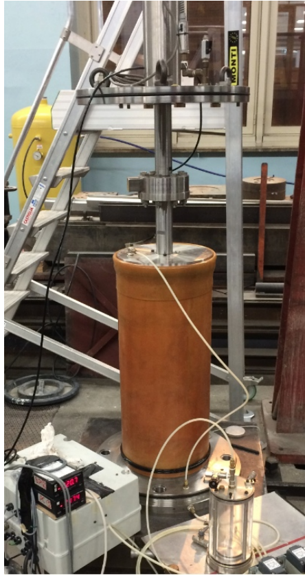
Figure 6.18: Dry sand sample with the external depression applied
