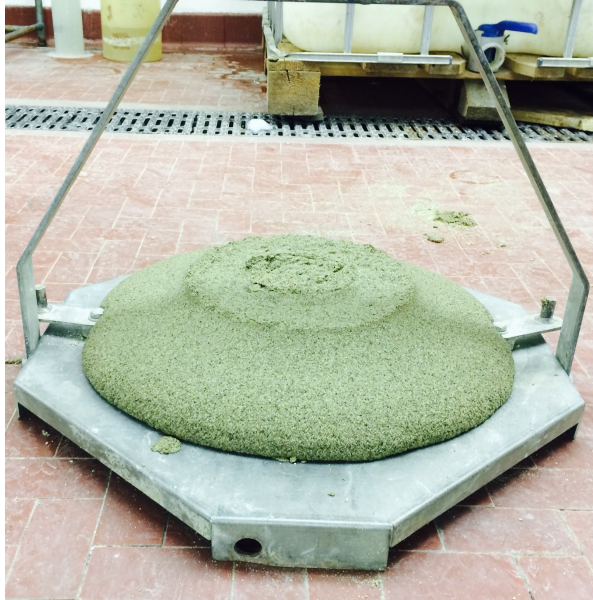
Figure 3.10: Optimal conditioning slump for Soil C
