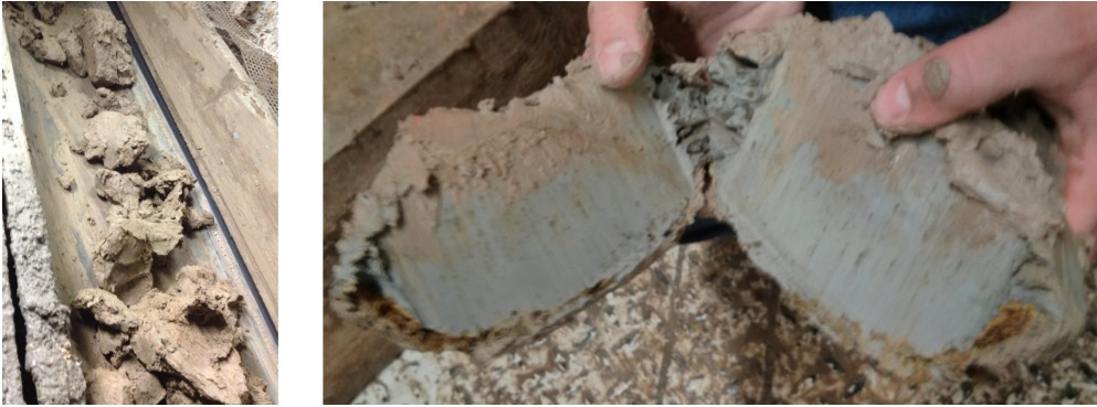
Figure 1.5: Example of clay chip sample as collected on the conveyor belt of an EPB machine excavating in a clay formation. The right picture clearly shows that the inner part of the chip is not conditioned and the conditioned mud is only outside the chip (Peila et al., 2015).
