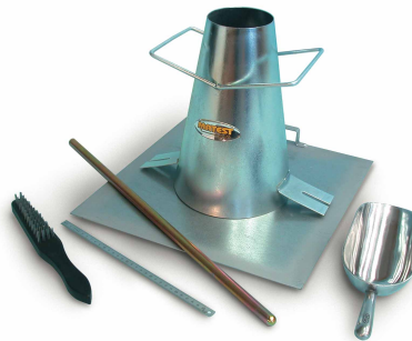
Figure 2.3: A standardized slump cone used for slump testing
