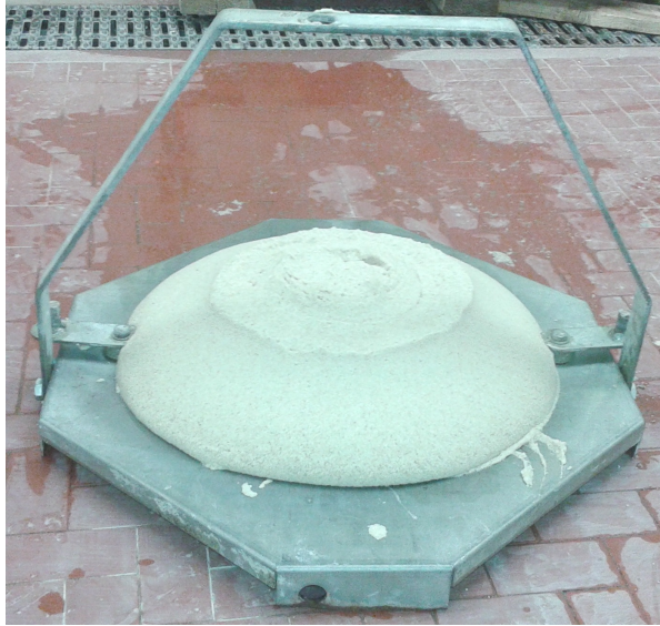
Figure 3.7: Optimal conditioning slump for Soil B
