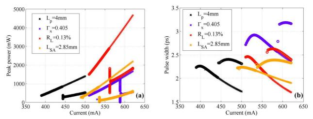
Figure 5 Bifurcation diagrams of the peak power (a) and the pulse width (b) for the four modified devices. These four devices are  $L_p = 4$  mm (black),  $\Gamma_x = 0.405$  (violet),  $R_L = 0.13\%$  (red) and  $L_{SA} = 2.85$  mm (yellow). For the sake of simplification, only the fundamental ML and the second harmonic ML branches are shown.
