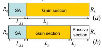
Figure 1 Schematic diagram of the considered two-section (a) and three-section (b) passively ML FP lasers in this paper.
