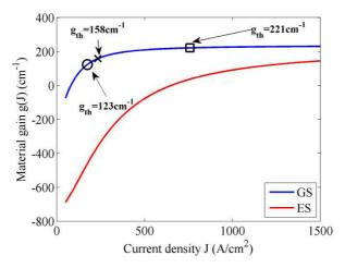
Figure 4 QD material gain as a function of the injection current density for the GS (blue line) and the ES (red line) of the considered device. The inserted first two markers indicate the threshold gain positions of the lasers without passive section (circle marker) and with a 4 mm long passive section (cross marker). The last square marker corresponds to a threshold gain position which will be discussed later.
