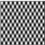
Figure 3. The Fourier components of 2D Fourier Transform are represented inside a plane. Several cases of signals in 2D are represented. The Fourier components might only lay on one axis (A), inside two quadrants (B), on both axis (C1), or all of the quadrants (C2) depending on the function used to generate the signal. In all cases, we can see that the Fourier components are symmetric through the origin (0,0) [5]. All signals extend from -\infty to \infty in both directions.
