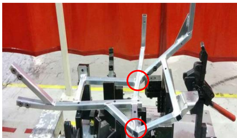
Figure 3 – Welding operation no. 30. Red circles show the corresponding weld areas.
