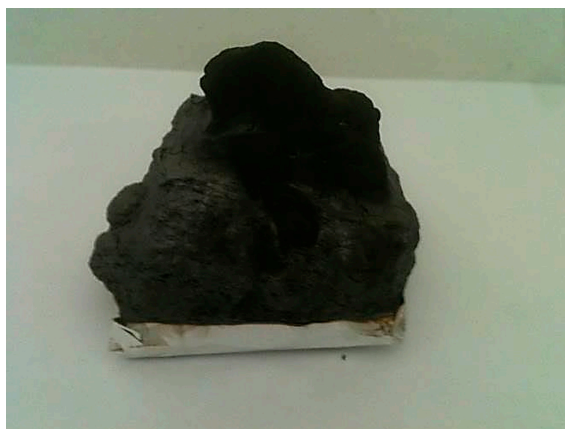
Figure 9. Residue of HT/E-15APP after cone calorimetry tests.
