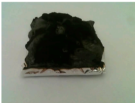
Figure 8. Residue of H/E-15APP after cone calorimetry tests.
