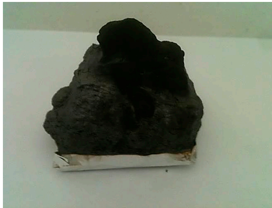
Figure 9. Residue of HT/E-15APP after cone calorimetry tests.
