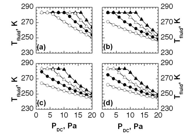
Design space of the selected product calculated at various values of dried layer thickness: (a)  $L_{dried}/L = 12\%$ ; (b)  $L_{dried}/L = 34\%$ ; (c)  $L_{dried}/L = 66\%$  and (d)  $L_{dried}/L = 99\%$ . ( $\bigcirc$ ) B type; ( $\bigcirc$ ) C type; ( $\triangle$ ) D and ( $\blacktriangle$ ) E type.
