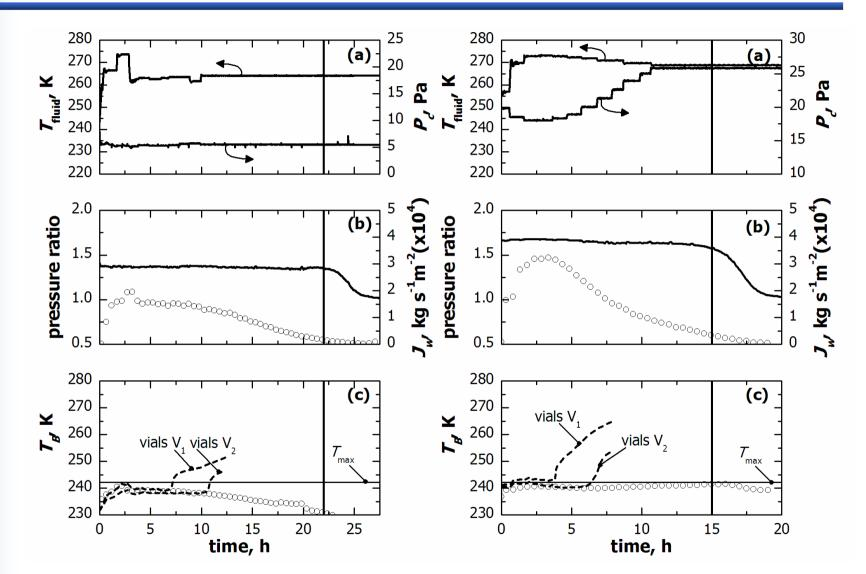
Freeze-drying cycles carried out using a 5% sucrose solution, and the MPC algorithm to manipulate only  $T_{\text{fluid}}$  and both  $T_{\text{fluid}}$  and  $P_{\text{c}}$ .
