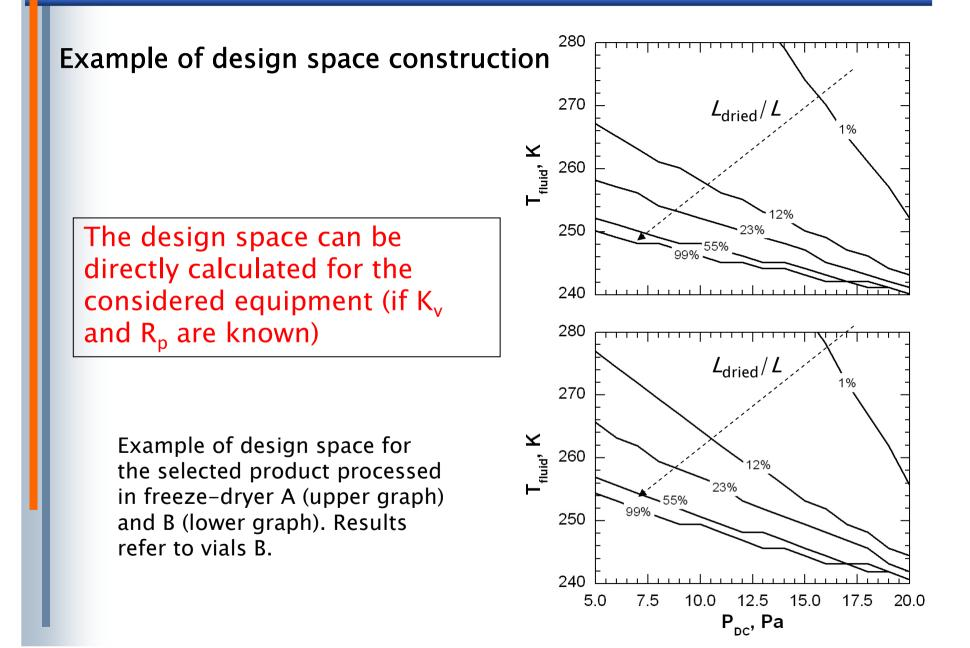
Recipe scale-up and optimisation in one test: In-line approach
