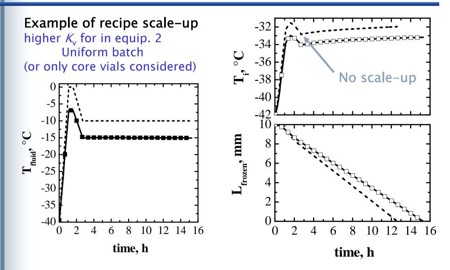
Comparison between the original recipe (dashed line) and the recipe calculate using the proposed scale-up algorithm (symbols). Evolution of the temperature at the interface of sublimation (upper graph) and of the thickness of the frozen layer (lower graph) in a vial in the first equipment (solid lines), and in the second equipment, when the original recipe is used (dashed lines) and when the scaled-up recipe is used (symbols).
