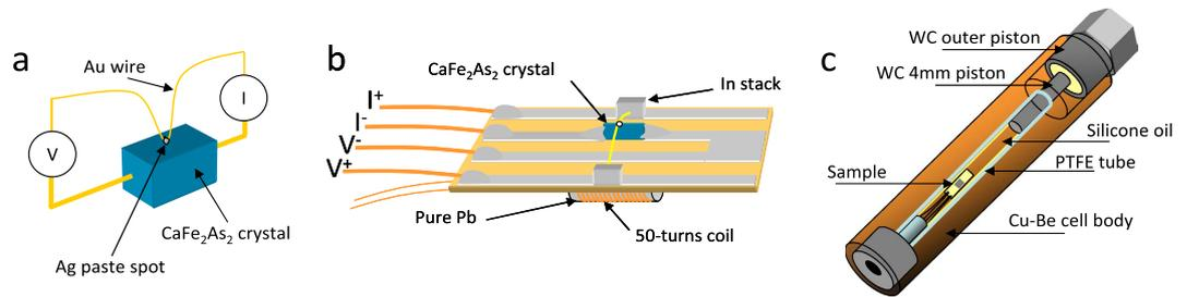
**Figure 1.** (a) Scheme of the “soft” point-contact technique, with the electric connections for PCARS measurements: A probe current  $I$  is injected into the crystal through the point contact and the voltage drop  $V$  across the contact is measured. (b) Drawing of the fiberglass board used as a sample holder. (c) Drawing of the Cu-Be pressure cell in which the sample is enclosed.
