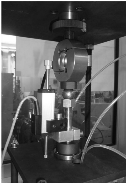
Figure 4.19 Detailed view of displacement transducer and load cell
