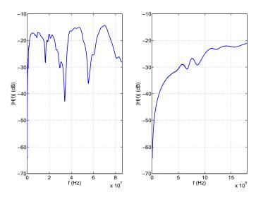
Fig. 1. Frequency-domain PLC channel response between the front right dipped headlight and the front left high beam. Left panel: [0, 86] MHz frequency range. Right panel: closeup on the [0, 1.8] MHz region.
