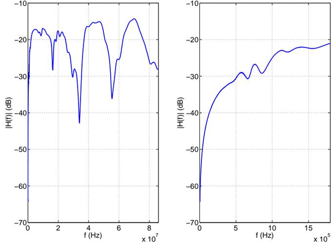
Fig. 1. Frequency-domain PLC channel response between the front right dipped headlight and the front left high beam. Left panel: [0, 86] MHz frequency range. Right panel: closeup on the [0, 1.8] MHz region.
