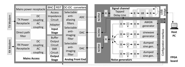
Fig. 5. Logic level architecture of the FPGA based channel emulator.
