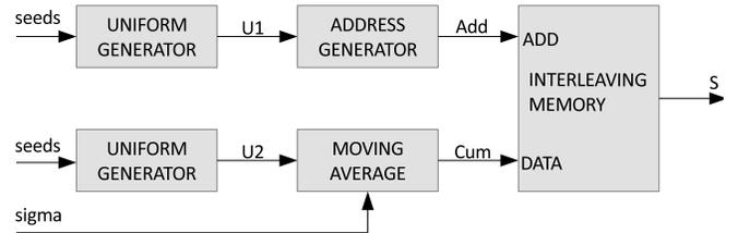
Fig. 7. Architecture of the AWGN generator.
