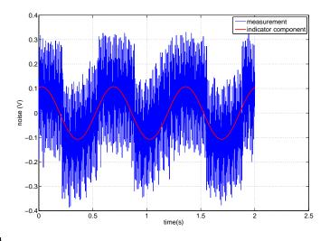
Fig. 3. Example of time-domain voltage measurement illustrating the effect of the very low frequency component (see text for details).
