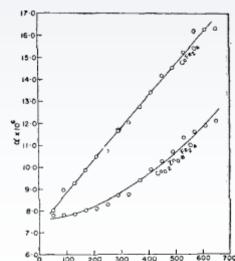
Temperature (\*C) FIG. I. Variation of the coefficient of thermal expansion of CoFe2O4 and Coa2na Fe2O4 with temperature.
