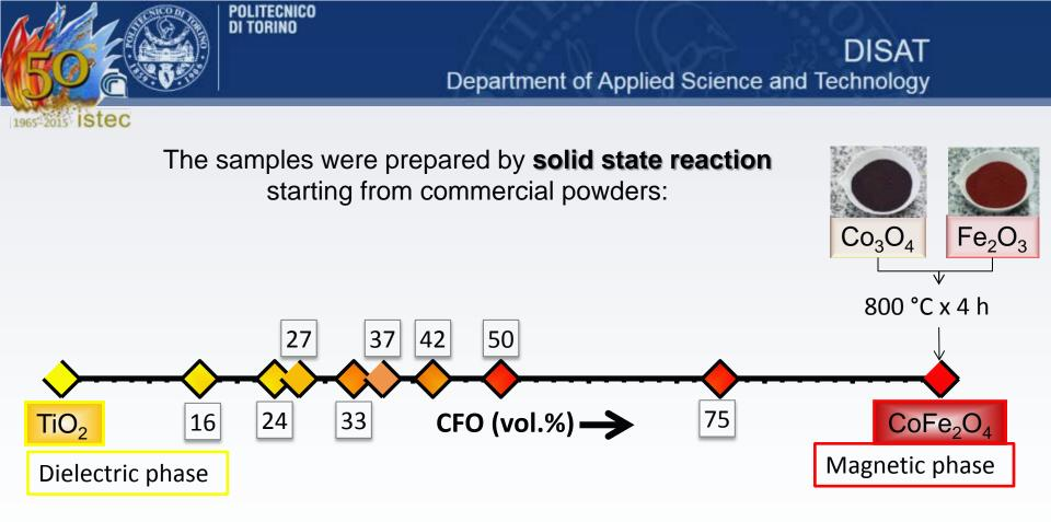
Sintered in air at 1200 °C for 2 h
