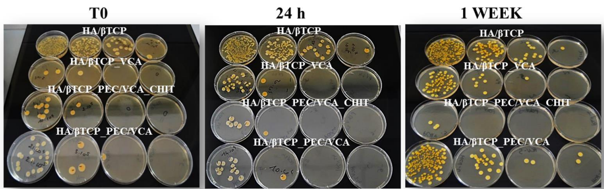
Figure 23. Images of Agar germ plate at time zero, after 24h and after 1 week. Photos shows the absence of CFU on Agar germ plate for HA/ \beta TCP_PEC/VCA_CHIT scaffold at already at low dilution of the starting solution.
