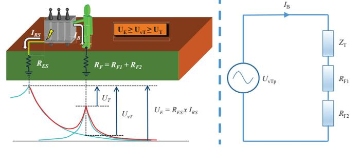
Figure 1. Increment of the permissible EPR ( $U_E$ ) due to the earth surface potential profile and additional resistances.  $I_B$  is the current flowing through the human body,  $Z_T$  is the total body impedance,  $R_{F1}$  is the resistance of the footwear,  $R_{F2}$  is the resistance to earth of the standing point.
