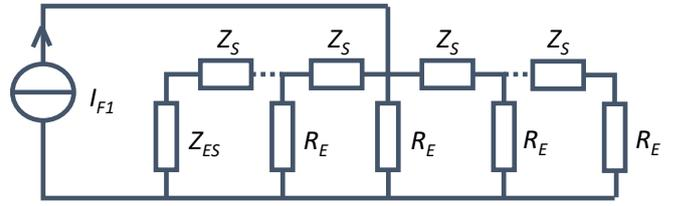
Figure 2. SLGF circuit model. The impedance  $Z_{ES}$  is the earth impedance of the HV/MV station;  $R_E$  is the average value of the MV/LV substation earth impedance;  $Z_S$  is the average value of the metal sheaths impedance.
