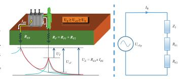
Figure 1. Increment of the permissible EPR  $(U_E)$  due to the earth surface potential profile and additional resistances.  $I_B$  is the current flowing through the human body,  $Z_T$  is the total body impedance,  $R_{F1}$  is the resistance of the footwear,  $R_{F2}$  is the resistance to earth of the standing point.
