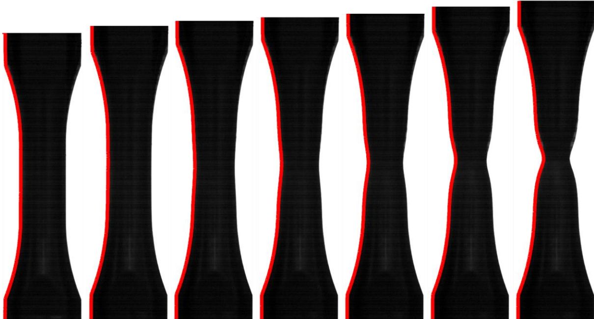
Fig. 1: Digital image elaboration for the edge identification (shape profile in red).
