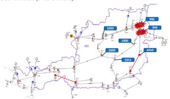
Fig. 5 Triggering events destroy 2 buses - 2 additional lines are studied as long-term countermeasures
