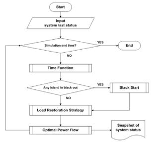
Fig. 3 High level flowchart of restoration optimal decision module
