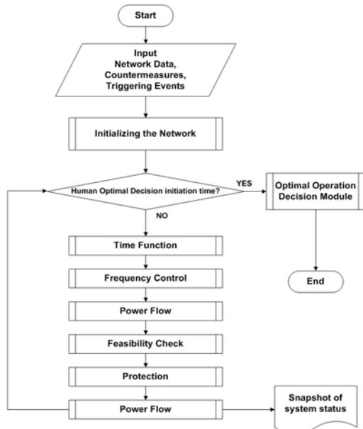
Fig. 2 High level flowchart of system automatic response
