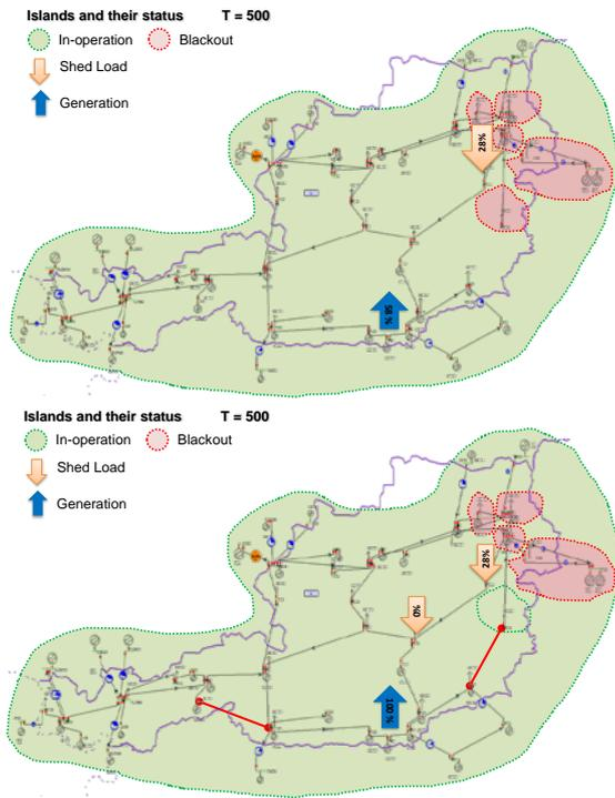
Fig. 8 Last snapshot – without and with invested lines
