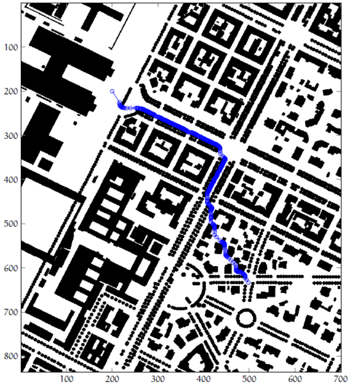
FIGURE 25 EXPERIMENT 1, SIMULATED EXPERIMENT. OBSTACLES FROM OPEN DATA ARE SHOWN AS BLACK CELLS; COMPUTED WAYPOINTS ARE SHOWN IN BLUE. THE STARTING POINT IS IN THE TOP-LEFT AND THE GOAL IN THE BOTTOM-RIGHT.
