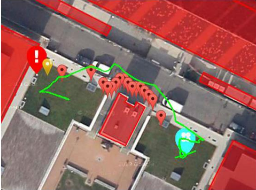
FIGURE 27 REAL TEST OVER A SHORT TRAJECTORY. OBSTACLES FROM OPEN DATA ARE SHOWN IN RED; STARTING POINT AND FINAL GOAL ARE SHOWN AS MARKERS; COMPUTED WAYPOINTS ARE SHOWN AS RED MARKERS. REAL TRAJECTORY FOLLOWED BY THE UAV IS SHOWN IN GREEN.
