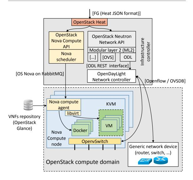
Figure 3.11: OpenStack-based Node.
