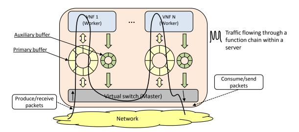
Figure 5.2: Deployment of the algorithm within a server.
