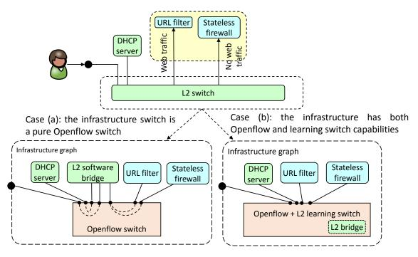
Figure 3.7: Example of the output of the reconciliation process when mapping a L2 switch functionality in case of two different types of infrastructure nodes.
