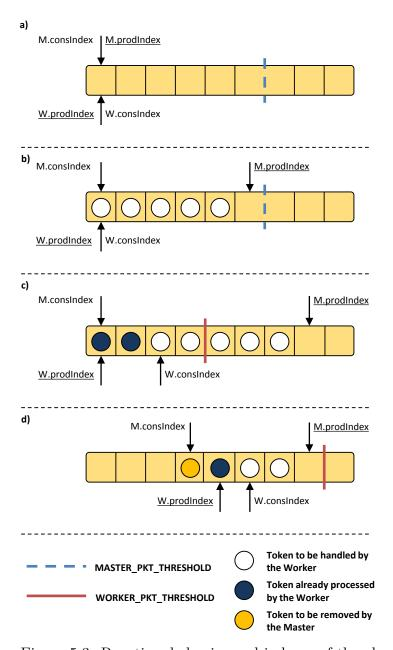
Figure 5.3: Run-time behavior and indexes of the algorithm.
