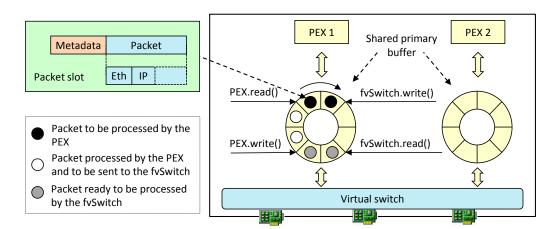
Figure 1.7: Packet exchange between the fvSwitch and PEX.
