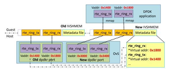
Figure 6.4: ivshmem device for port remapping.
