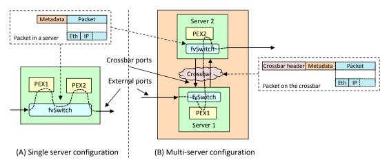
Figure 1.8: Single vs. multi-server architecture.
