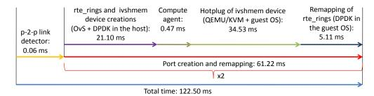
Figure 6.10: Time required to establish a direct connection.
