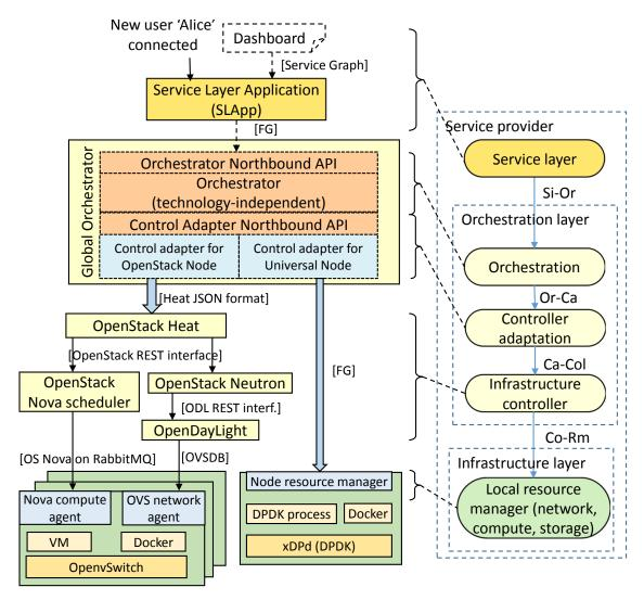
Figure 3.2: Overall view of the system, including the two implementations of the infrastructure layer.
