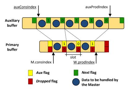
Figure 5.4: Binding primary buffer - auxiliary buffer.
