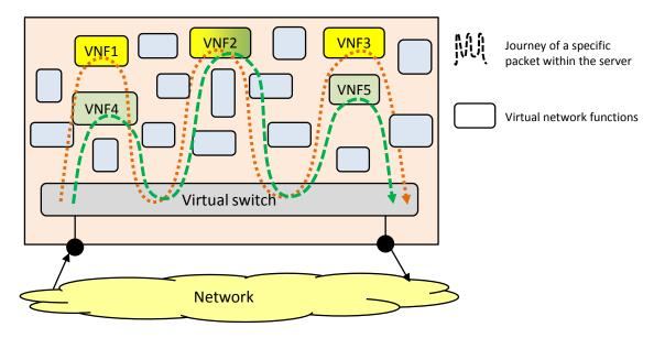
Figure 5.1: Function chains deployed in a server.
