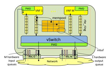
Figure 4.3: Implementation that exploits the FDIR feature.
