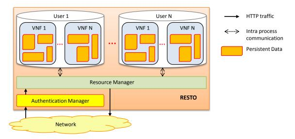
Figure 2.2: Internal view of the Remote Storage Service.
