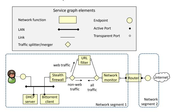
Figure 3.3: Service graph: basic elements and example.
