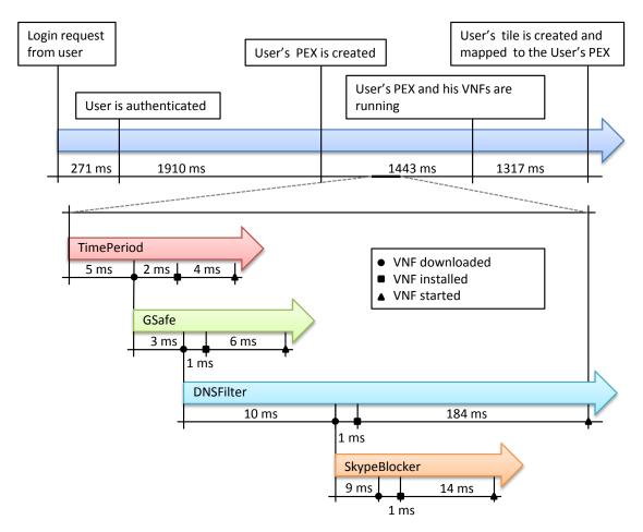
Figure 2.5: Starting a PEX with four VNFs.
