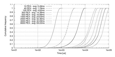
Figure 1.10: Latency introduced by the node with a growing number of native PEX.
