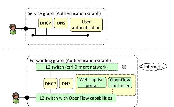
Figure 3.9: Authentication SG and FG.
