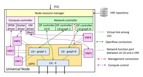
Figure 3.10: Logical architecture of the Universal Node.
