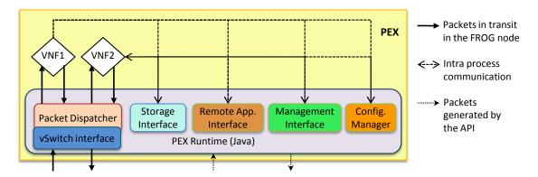
Figure 2.4: Exploded view of a PEX hosting two VNFs.
