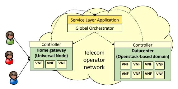
Figure 3.1: Deployment of virtual network functions on the telecom operator network.
