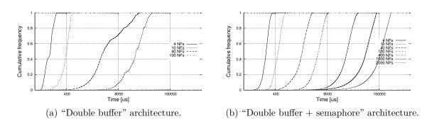
Figure 4.5: Latency introduced by the framework.
