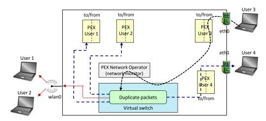
Figure 1.4: Possible journey of a broadcast/multicast packet.
