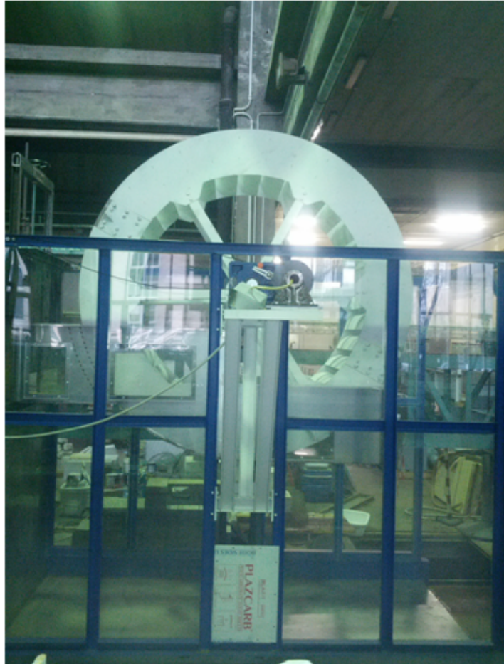
Fig. 3. The installed wheel in 2.12 m in diameter and 32 blades. At the shaft axis the gearbox and the generator are visible.
