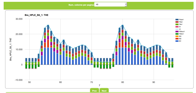
Fig. 6. Power profiles (hot water energy vector) of the components in week 1 for Configuration 1.
