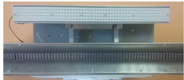
Figure 8. Receiving antenna (50 cm long) designed realized in microstrip on top of a portion of the transmitting slotted waveguide antenna.
