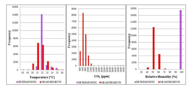
Fig. 2. Temperature, CO<sub>2</sub> concentration, relative humidity comparison between measurements and simulated value of deterministic scenario.
