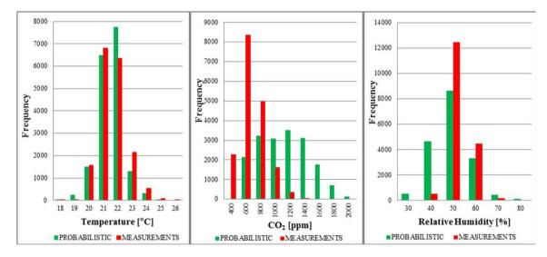
Fig. 5. Temperature, CO<sub>2</sub> concentration, relative humidity comparison between measurements and simulated value of probabilistic scenario
