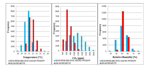
Fig. 3. Temperature, CO2 concentration, relative humidity comparison between measurements and simulated value of semi-probabilistic scenario (influence of window opening and closing behaviour).
