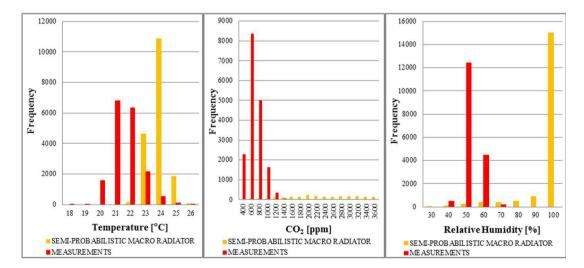
Fig. 4. Temperature, CO<sub>2</sub> concentration, relative humidity comparison between measurements and simulated value of semi-probabilistic scenario (influence of heating set-point adjustment).
