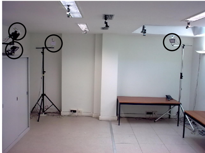
Figure 1. MScMS-II prototype. (a) Sensor network configuration: black circles highlight the spatial position of the network nodes.
