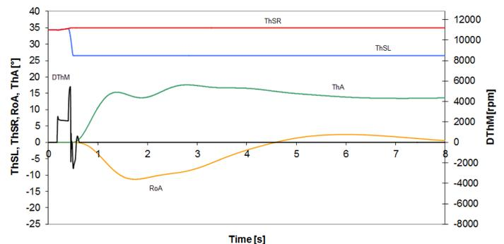
Fig. 16 Flaps deployment under high load – technique 2d
