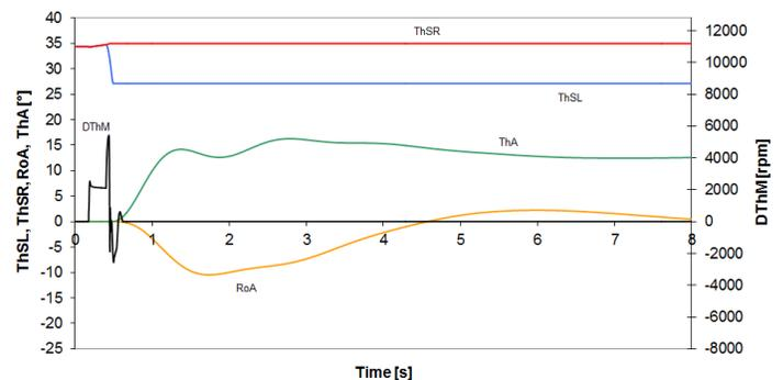
Fig. 15 Flaps deployment under high load – technique 2c
