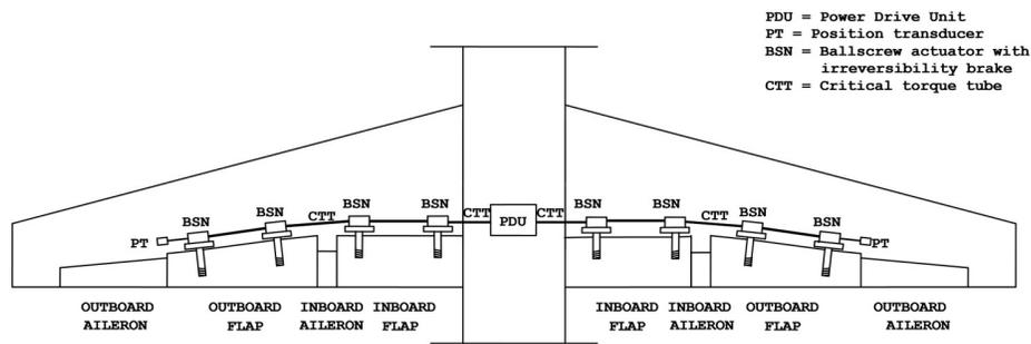
Fig. 2: No-Back Irreversibility Brakes (NBB) Flap Architecture
