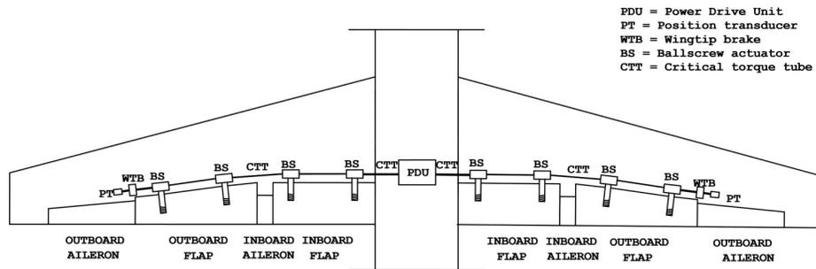
Fig. 1 Wing tip Brakes (WTB) Flap Architecture.
