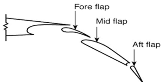
Fig. 3 Schematic Diagram for Triple Slotted Flap
