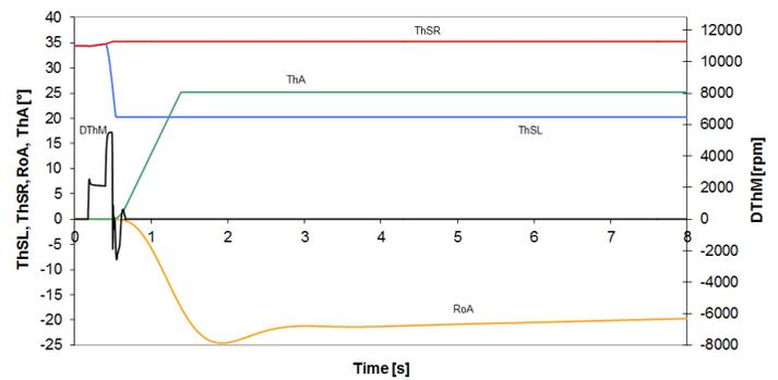
Fig. 13 Flaps deployment under very high load – technique 1
