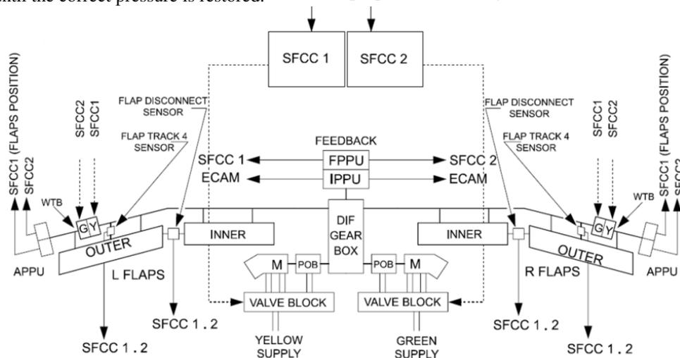
Fig. 5 Schematic of A330 Flap Actuation System
