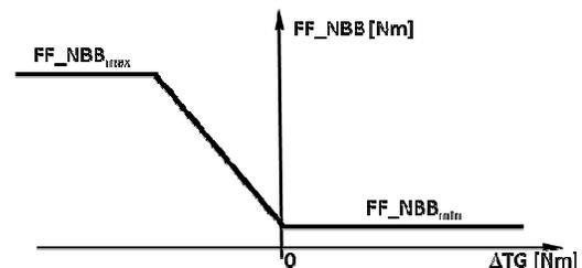
Fig.10 NBB Braking Torque as a function of  $\Delta TG$
