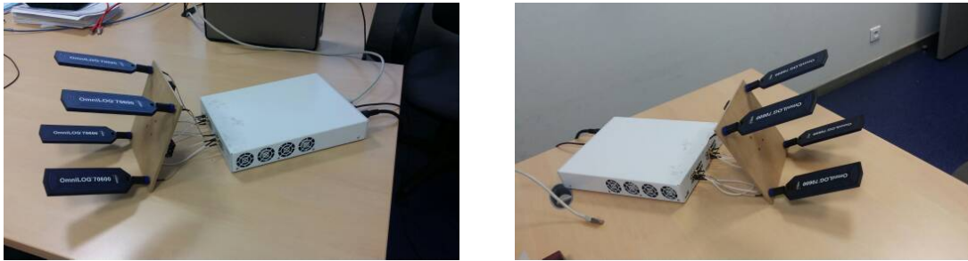
Figure 11.6: Nutaq PicoSDR 4x4 with 4 Aaronia OmniLOG 70600 antennas.
