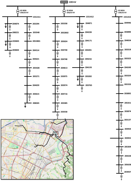
Fig. 3 The portion of MV distribution grid for the demo simulation
