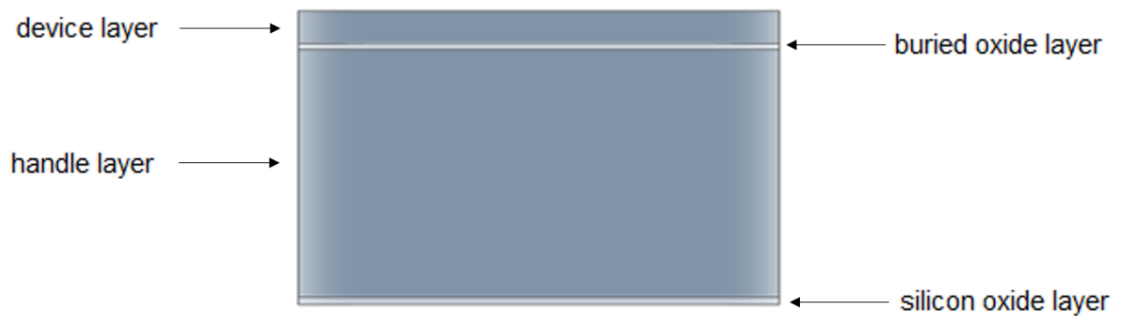
Fig. 2.1. Cross-sectional view of the SOI wafer used for the cantilever fabrication.
