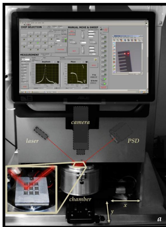
Fig. 2.6. A photograph of the measurement set-up and a close view of the holding cell.
