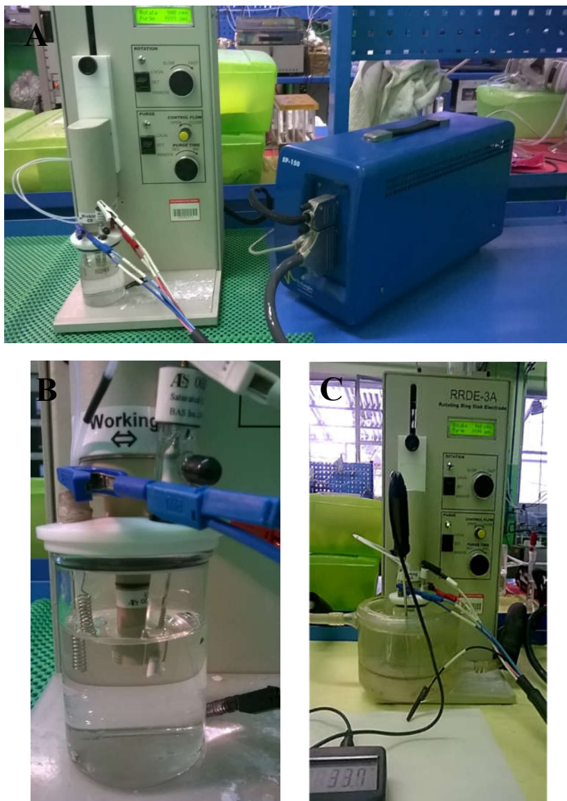
Figure 17. (A) RDE experimental setup for ORR tests in Politecnico di Torino – Green 2 Group Laboratory: RDE apparatus (Mod. ALS RRDE-3A) + Potentiostat (Mod. Bio-Logic SP-150). (B) Detail of the RDE 3-electrode electrochemical cell. (C) RDE apparatus coupled with thermostatic bath vessel used for measurement at different temperatures.
