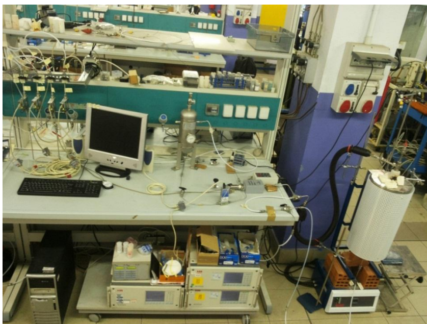
Fig.2.12: Picture of the lab-scale rig with vertical furnace
