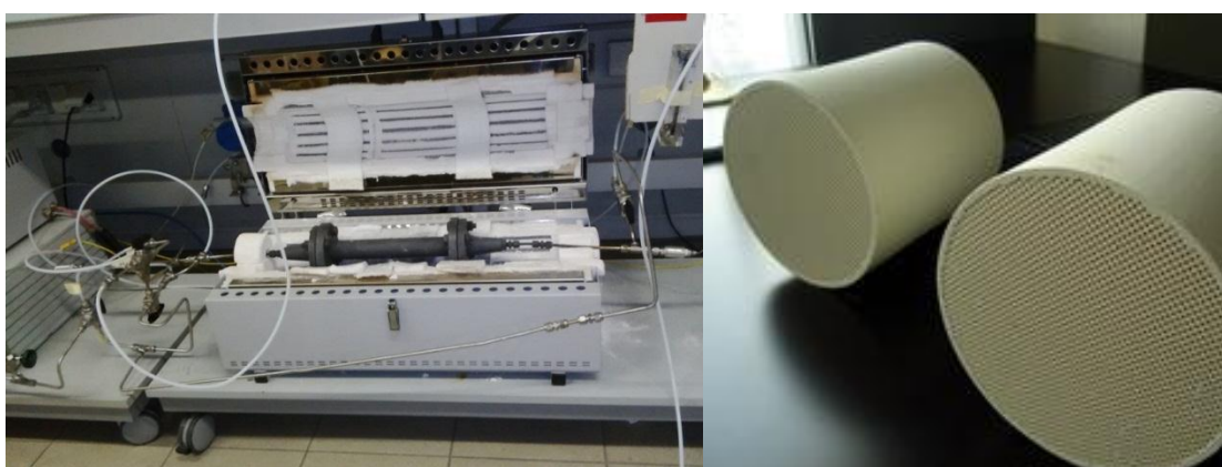
Fig.2.13: Picture of the oven with canning (left) and the honeycomb monoliths (right)
