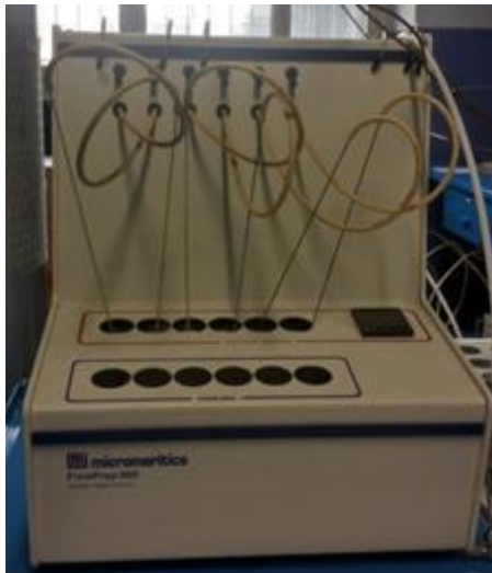
Fig. 2.2: Pretreatment equipment for removing pollutants
