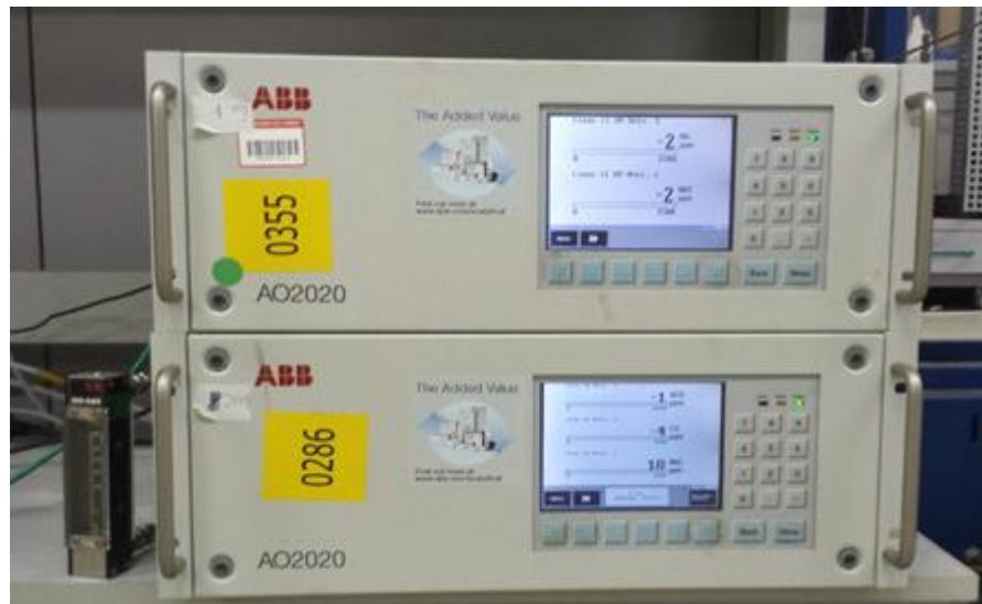
Fig. 2.14: UV gas analyser Limas (above), gas analyser Uras (below) and flow meter (left)
