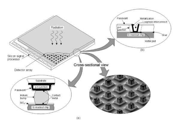
Figure 1.6. Hybrid IR FPA with independently optimized signal detection and readout: (a) indium bump technique; (b) loophole technique. The figure is from [11].
