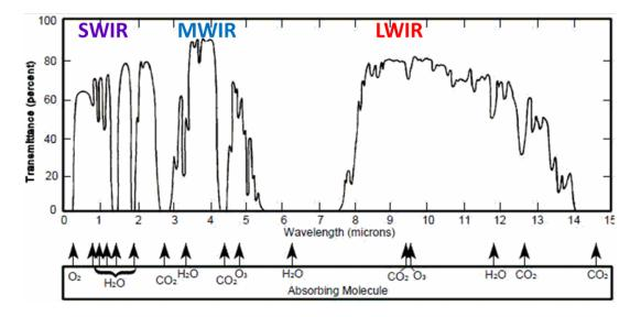
Figure 1.1. Atmospheric transmittance of electromagnetic radiation vs. wavelength.
