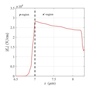
Figure 4.6. Calculated vertical component of the electric field  $|\mathcal{E}_z|$  in set A near the *p*-*n*<sup>-</sup> junction (marked with a vertical dashed line) at a bias  $V_{\text{bias}} = -3$  V.
