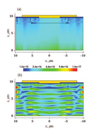
Figure 5.10.  $A_{\text{opt}}$  distribution (cm<sup>-3</sup>s<sup>-1</sup>) obtained with (a) ray tracing and (b) FDTD, across the vertical symmetry plane shown in Fig. 5.1, for  $t_{\text{abs}} = 9.5 \,\mu\text{m}$ ,  $a_{\text{CdTe}} = 6 \,\mu\text{m}$ ,  $W_{\text{met}} = 16 \,\mu\text{m}$  at  $\lambda = 9.1 \,\mu\text{m}$ .
