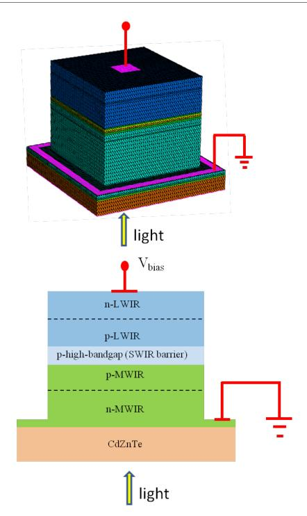
Figure 3.8. 3D (above) and 2D (below) structure of the dual-band single-pixel detector.
