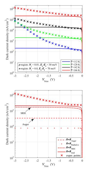
Figure 4.4. Set A: simulated  $J_{\text{dark}}(V;T)$  (above) and corresponding components at T = 166 K (below). Crosses indicate experimental values.
