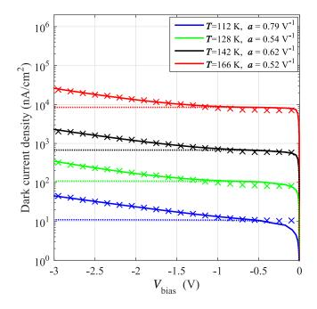
Figure 4.8. Set B: simulated  $J_{dark}(V;T)$  considering the contributions of Auger, SRH and radiative GR (dotted lines), and with the further inclusion of I.Ion. (solid lines). Crosses indicate experimental values. BTBT is not required to obtain a satisfactory agreement with experiments.
