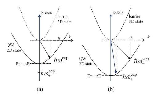
Figure 6.12. Capture scattering scheme from a parabolic  $E_k$  bulk barrier state (dashed) to a quantum well state (solid) with a binding energy  $\Delta E$ . (a) No capture is possible via phonon-plasmon emission with frequency  $\omega_+^{cap}$ , whereas capture via the  $\omega_-^{cap}$  mode is allowed with the emission of a phonon-plasmon of momentum  $q_{\parallel}$ . (b) In this case the capture is possible through both plasmon modes.
