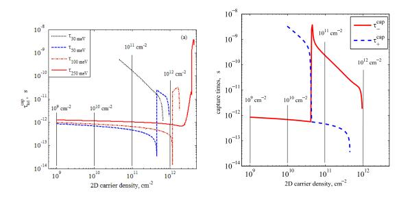
Figure 6.14. (a) Total capture time versus 2D carrier density, for several values of quantum well state binding energy (30, 50, 100 and 250 meV). (b) Capture times  $\tau_{-}^{cap}$  and  $\tau_{+}^{cap}$  versus carrier density (respectively via  $\omega_{-}^{cap}$  and  $\omega_{+}^{cap}$ ) for  $\Delta E = 50$  meV. The vertical black lines correspond to density values as in Fig. 6.13.
