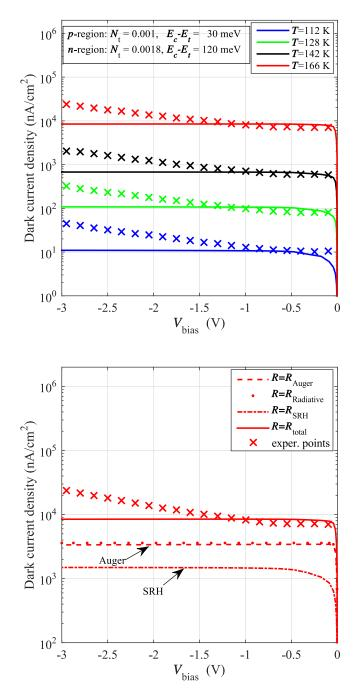
Figure 4.5. Set B: simulated  $J_{\text{dark}}(V;T)$  (above) and corresponding components at T = 166 K (below). Crosses indicate experimental values.
