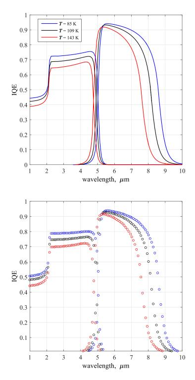
Figure 3.10. Dual-band detector: 3D (above, solid lines) and 2D (below, symbols) IQE for three values of T.
