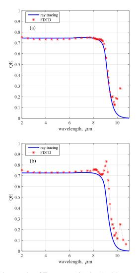
Figure 5.5. Second example: QE spectra, simulated with ray tracing and FDTD, for  $t_{abs} = 9.5 \,\mu\text{m}$ ,  $a_{CdTe} = 6 \,\mu\text{m}$ . (a)  $W_{met} = 11 \,\mu\text{m}$ , (b)  $W_{met} = 16 \,\mu\text{m}$ .
