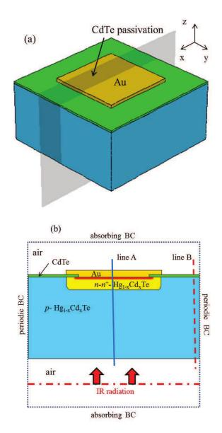
Figure 5.1. (a) 3D single pixel geometry and (b) 2D cut along a vertical symmetry axis. The vertical lines (A, B) mark the 1D cuts along which interesting quantities are plotted in the following. The computational box (dotted line) and optical boundary conditions are also shown.
