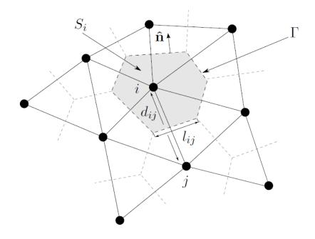
Figure 1.10. Schematic representation of a "box-method" grid. The dashed shapes are the edges of the finite boxes and are calculated through the bisectors of the triangle sides converging in the corresponding *node*. The grey area represents the finite box surrounding the *i*-th node.
