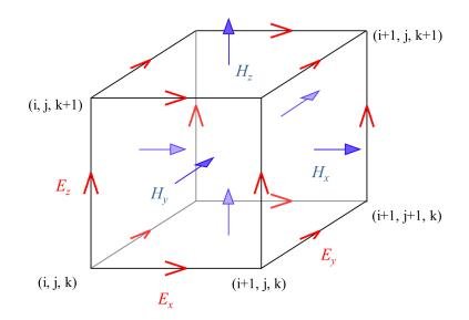
Figure 5.2. Schematic representation of the Yee grid [90]. The position of the electric and magnetic fields in relation to each other implicitly enforces the boundary conditions contained in Maxwell's equations. The electric and magnetic fields are solved at alternating grid points in space.
