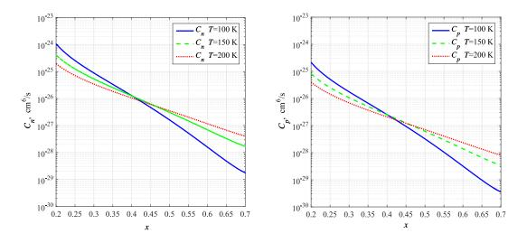
Figure 2.7. Auger electrons recombination coefficients as functions of Cd molar fraction x.
