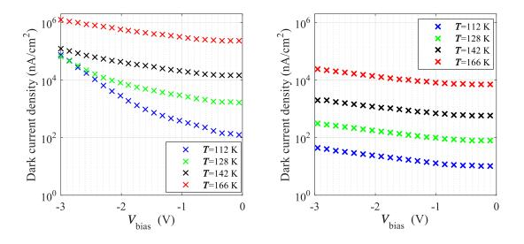
Figure 4.3. Experimental  $J_{dark}(V;T)$  for set A (left) and set B (right).
