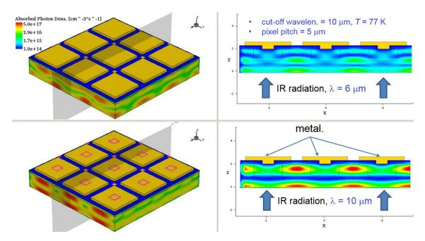
Figure 5.11.  $A_{\rm opt}$  obtained with FDTD, for a  $3 \times 3$  LWIR pixel array with 5  $\mu$ m pixel pitch (preliminary design).
