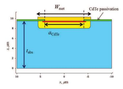
Figure 5.3. Geometrical parameters considered in the present study: absorber thickness  $t_{abs}$ , CdTe aperture  $a_{CdTe}$ , metallization width  $W_{met}$ .
