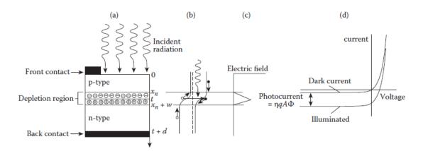
Figure 1.4. p - n junction photodiode: (a) structure of abrupt junction, (b) energy band diagram, (c) electric field, and (d) current-voltage characteristics for the illuminated and nonilluminated photodiode. The figure is from [8, Ch. 9].
