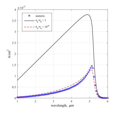
Figure 3.5. 1D analysis of the photocurrent spectrum for the single-color MWIR HgCdTe photodetector at T = 85 K,  $V_{\text{bias}} = 0.2$  V, with an illumination of 1 mW/cm<sup>2</sup>: numerical simulation (blue symbols), closed-form calculations with uniform (black solid) and exponential (red dashed) lifetime law, with  $L_0 = L/1.5$ .
