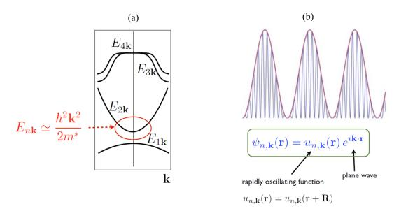
Figure 6.1. (a) Band structure around the  $\Gamma$  point for a typical direct band bap semiconductor. (b) Eigenfunctions of the Hamiltonian operator (electron in the ionic periodic potential).
