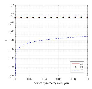
Figure 3.4. Single-color detector: 3D, 2D and 1D simulation of the minority carrier lifetime near the illuminated face at T = 85 K and  $V_{\text{bias}} = 0.2$  V, with an illumination of 1 mW/cm<sup>2</sup> at  $\lambda = 5 \,\mu$ m.
