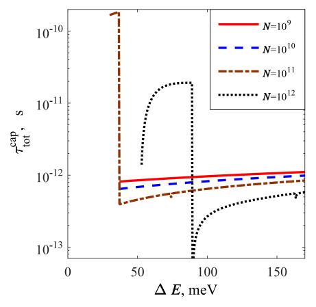
Figure 6.13. Total capture time versus quantum well binding energy, for several values of 2D carrier density N (in the legend, values are in cm<sup>-2</sup>).
