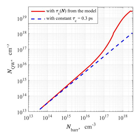
Figure 7.3. Carrier density  $N_{\text{QW}}$  versus  $N_{\text{barr}}$  for the QW considered in [137], calculated with the density-dependent capture time  $\tau_{c,ph}$  (red solid line) and with a fixed capture time  $\tau_{c,0} = 0.3$  ps (blue dashed line).
