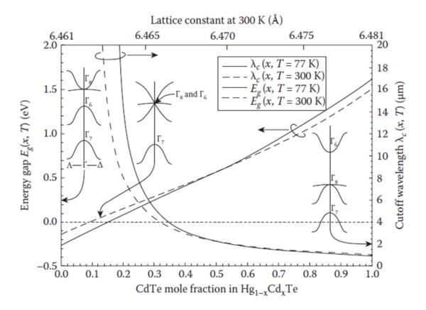
Figure 2.1. The bandgap structure of  $Hg_{1-x}Cd_xTe$  near the  $\Gamma$ -point for three different values of the forbidden energy gap. The energy bandgap is defined at the difference between the  $\Gamma_6$  and  $\Gamma_8$  band extrema at  $\Gamma = 0$  (figure from [8, Ch. 14]).
