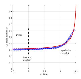
Figure 4.2. SIMS profile (blue symbols) of the Cd mole fraction x near the surface (located at  $z = 8.5 \,\mu\text{m}$ ) and least-squares fit (red solid line) used in the simulations. The estimated position of the p- $n^-$  junction is marked with a vertical dashed line.
