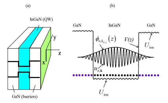
Figure 6.2. (a) InGaN/GaN typical heterostructure scheme. (b) electronic Bloch's state state in the QW. The dots represent the ionic lattice.
