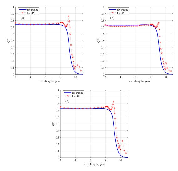
Figure 5.6. Third example: QE spectra, simulated with ray tracing and FDTD, for  $t_{abs} = 9.5 \,\mu\text{m}$ ,  $W_{met} = 16 \,\mu\text{m}$ . (a)  $a_{CdTe} = 2 \,\mu\text{m}$ , (b)  $a_{CdTe} = 4 \,\mu\text{m}$ , (c)  $a_{CdTe} = 6 \,\mu\text{m}$ .
