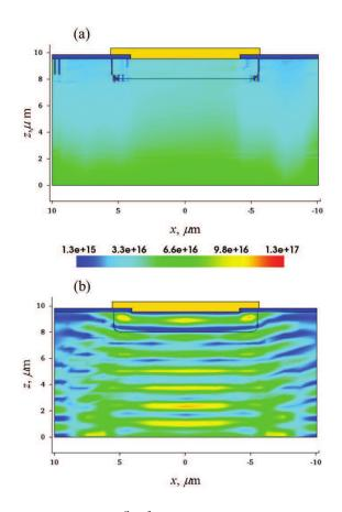
Figure 5.7.  $A_{\text{opt}}$  distribution (cm<sup>-3</sup>s<sup>-1</sup>) obtained with (a) ray tracing and (b) FDTD, across the vertical symmetry plane shown in Fig. 5.1, for  $t_{\text{abs}} = 9.5 \,\mu\text{m}$ ,  $a_{\text{CdTe}} = 6 \,\mu\text{m}$ ,  $W_{\text{met}} = 11 \,\mu\text{m}$  at  $\lambda = 9 \,\mu\text{m}$ .
