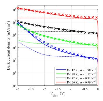
Figure 4.7. Set A: simulated  $J_{dark}(V;T)$  considering the contributions of Auger, SRH and radiative GR and BTBT (dotted lines), and with the further inclusion of I.Ion. (solid lines). Crosses indicate experimental values.
