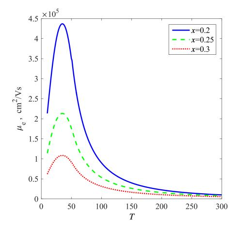
Figure 2.5. Electron mobility as a function of temperature.
