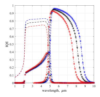
Figure 3.11. Dual-band detector: 1D simulation of IQE for three values of T, variant A (symbols) and variant B (dashed lines).
