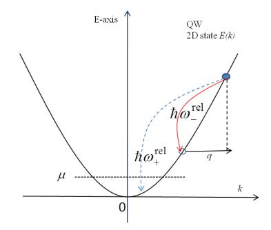
Figure 6.9. Relaxation of an electron with energy E(k) by the emission of a phonon-plasmon. In the example, the mode  $\omega_{-}^{rel}$  (blue solid arrow) is allowed, whereas  $\omega_{+}^{rel}$  (red dashed) is forbidden.
