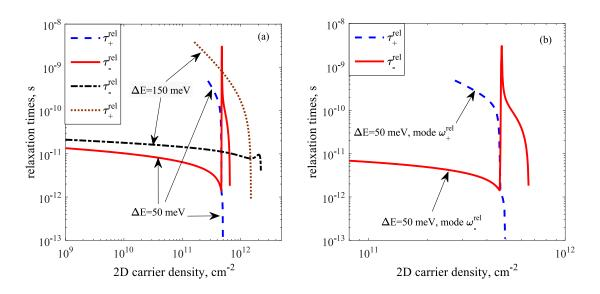
Figure 6.11. (a) Relaxation times  $\tau_{-}^{\text{rel}}$  (solid and dash-dotted lines) and  $\tau_{+}^{\text{rel}}$  (dashed and dotted lines) for an electron in a confined state of a 8 nm wide quantum well, with a kinetic energy respectively of E(k) = 50 and 150 meV. (b) Detail of the case for E(k) = 50 meV, showing the exchange of the two modes.
