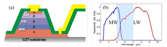
Figure 1.7. (a) Schematic of dual-band MWIR / LWIR detector pixel; (b) its experimental normalized spectral response spectrum at about 60 K. The cut-off wavelengths of the two bands were 5.4  $\mu$ m for the MWIR and 9.1  $\mu$ m for the LWIR band. The figure is from [13].
