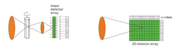
Figure 1.5. First (left) and second (right) generation of FPAs.
