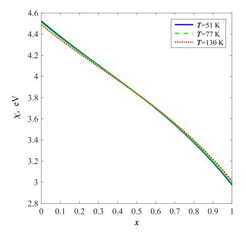
Figure 2.4. Electron affinity as a function of Cd molar fraction x.
