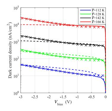
Figure 4.9. Set B: simulated  $J_{dark}(V;T)$  considering the contributions of Auger, SRH and radiative GR, and either I.Ion. (solid lines) or TAT (dashed lines). The *T*-dependence of experimental characteristics (symbols) can be reproduced with I.Ion., not with TAT.
