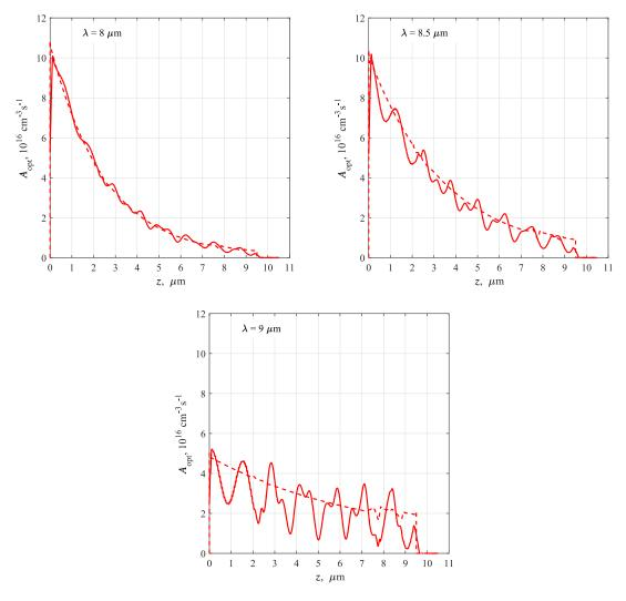
Figure 5.9.  $A_{opt}$  obtained with ray tracing (dashed lines) and FDTD (solid lines) along line B (see Fig. 5.1(b)), for  $\lambda = 8, 8.5, 9 \,\mu$ m.
