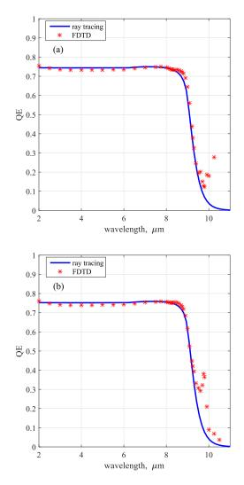
Figure 5.4. First example: QE spectra, simulated with ray tracing and FDTD, for  $W_{\text{met}} = 11 \,\mu\text{m}$ ,  $a_{\text{CdTe}} = 6 \,\mu\text{m}$ . (a)  $t_{\text{abs}} = 9.5 \,\mu\text{m}$ , (b)  $t_{\text{abs}} = 10.5 \,\mu\text{m}$ .
