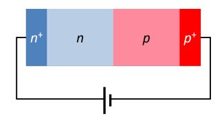
Figure 1.8. Schematic of HOT detector.
