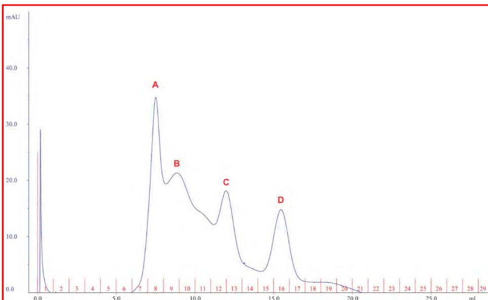
Figure 5.48: Size-exclusion chromatograms of M1 mutant purification.
