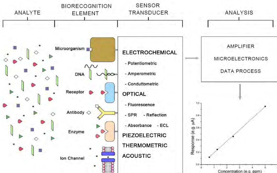
Figure 2.1: General scheme of a biosensor.
