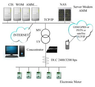
Figure 2. Telegestore system architecture
