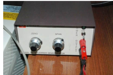
Figure A.10: Demodulator.
