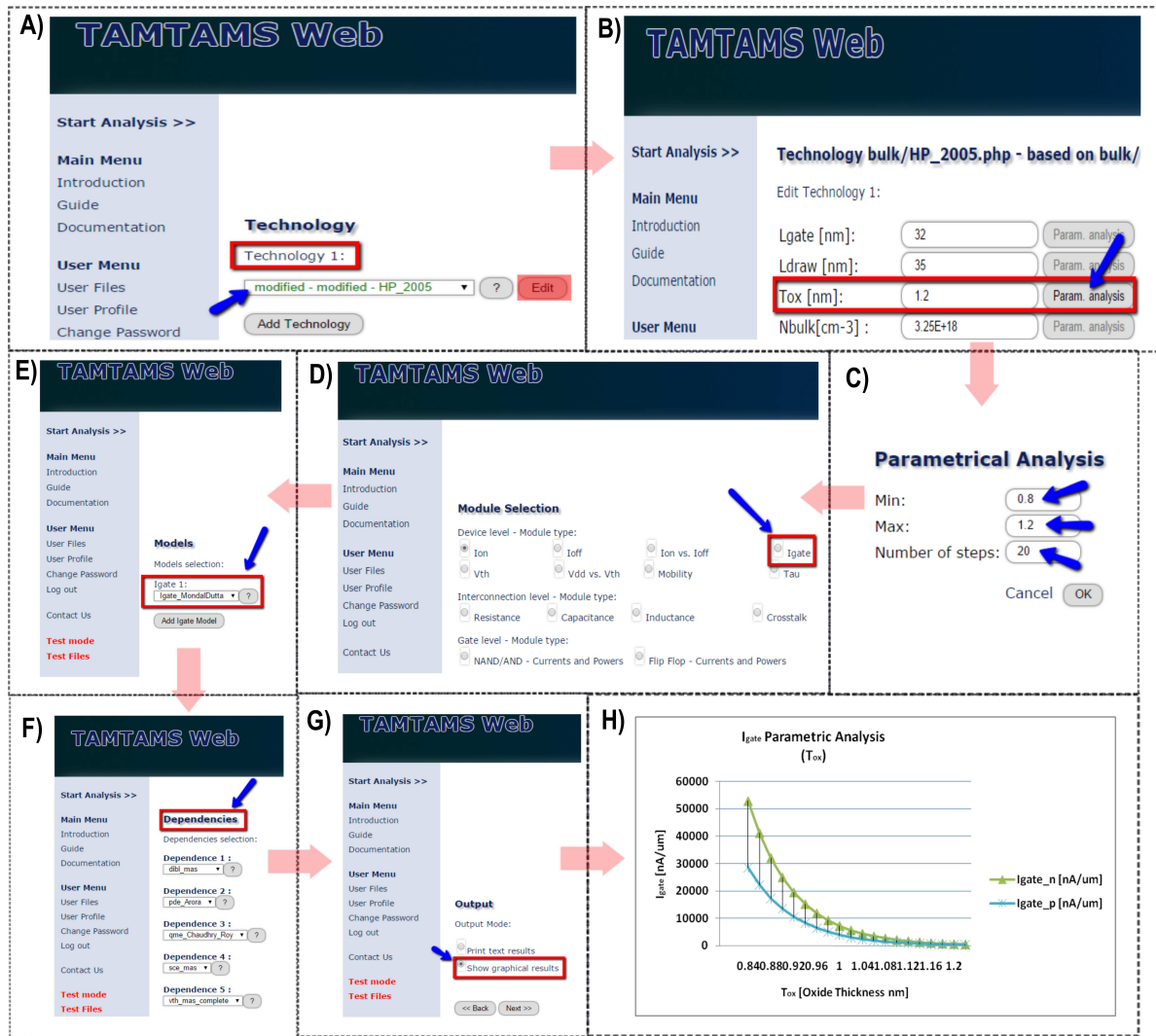
Fig. 8. Case of study. Igate parametric analysis choosing one specific technology node and varying the oxide thickness. A) Technology selection. B) Choice of the parameter to be changed. C) Setting of the parameter range to be used in the analysis. D) Module selection. E) Model selection. F) Dependencies selection. G) Output type selection. H) Output result.
