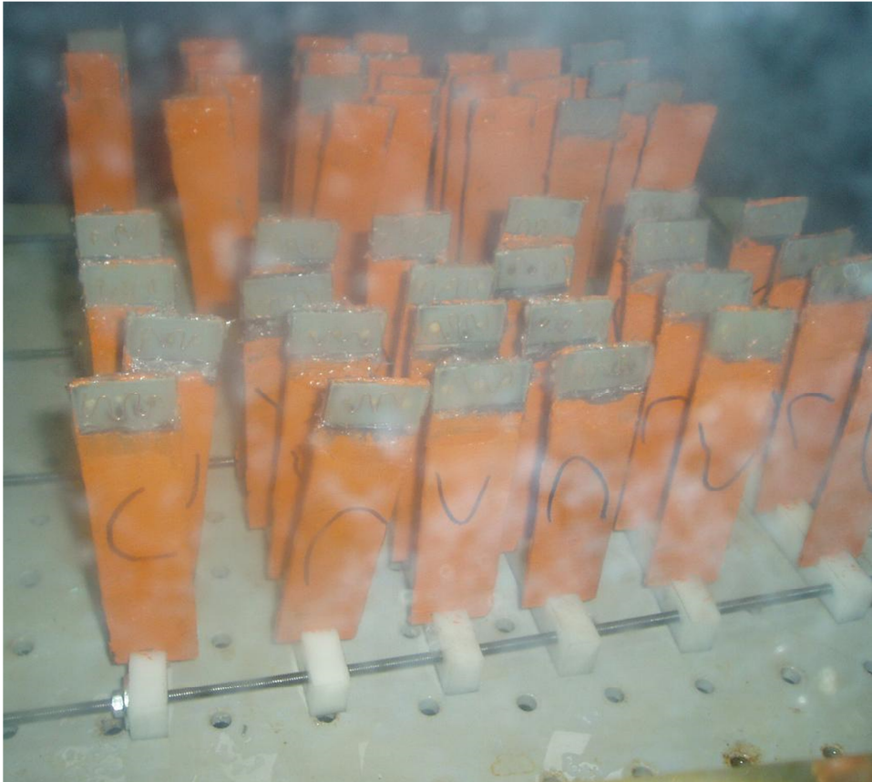
Fig. 4. Open-faced specimens during exposure to humid and warm environment.
