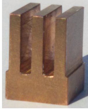
Figure 2: Reference heat sink.
