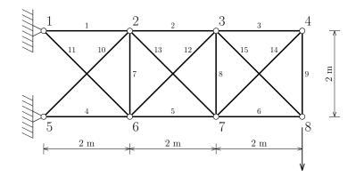
Figure 1: Schematic of the truss used in the analysis. The nodes and the rods are numbered.
