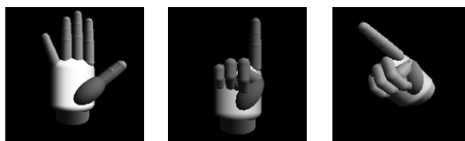
Figure 5. 3D hand model used for generating the reference poses (three configurations are shown, obtained by working on a subset of the possible DOFs).
