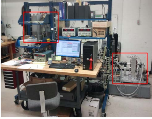
Figure 7. View of the test rig. The dSPACE 1103 PPC host computer is on the desk. The machine-under-test is in the red square to the right, connected to an induction machine dyno via an inline torquemeter (not visible). The red square to the left identifies the power converters.
