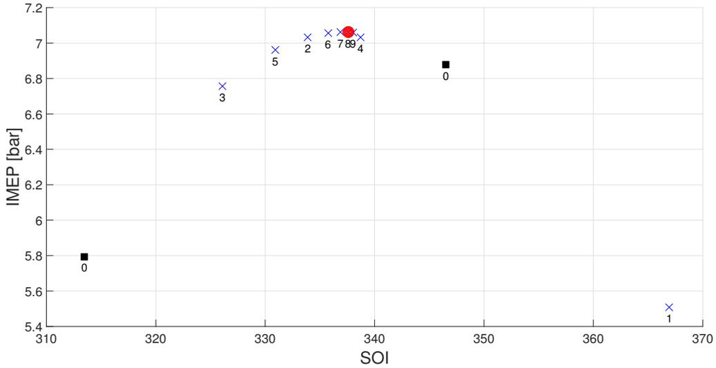
Figure 4.5: Iterations of the golden section search method.
