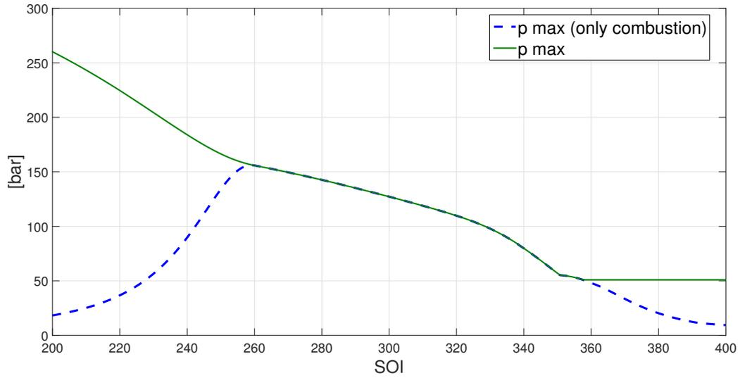
Figure 3.6: The peak firing pressure  $p_{\max}$  for different values of SOI, taking into account only combustion (blue curve) or the absolute maximum (green curve),
