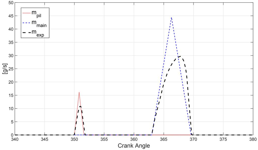
Figure 3.1: Pilot and main injections @1500x5 engine point
