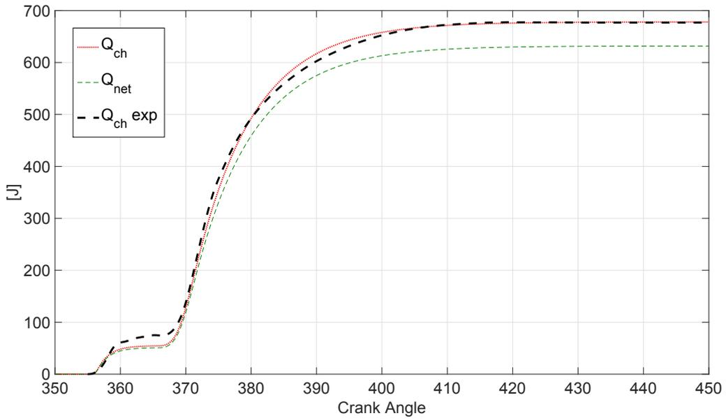
Figure 3.2:  $Q_{ch}$ , and  $Q_{net}$  @1500x5 engine point
