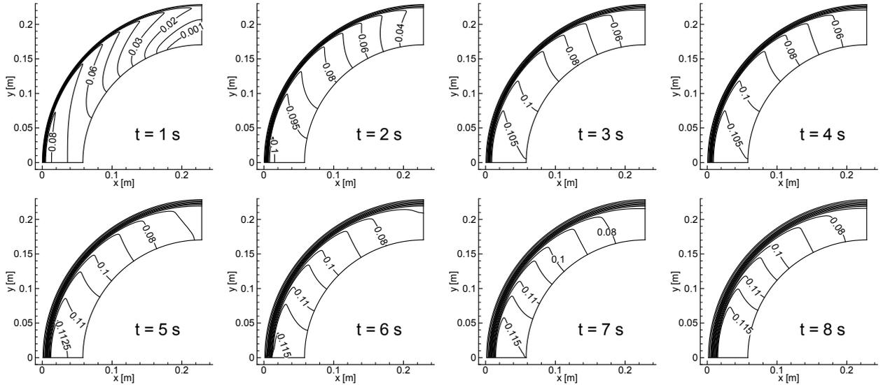
(b) Pyrolysis gas density,  $\rho_g$  [kg/m<sup>3</sup>], at different times.
