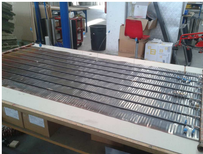
Figure 11 Full scale prototype: thermocouples inserted inside the thermal collector pipes.
