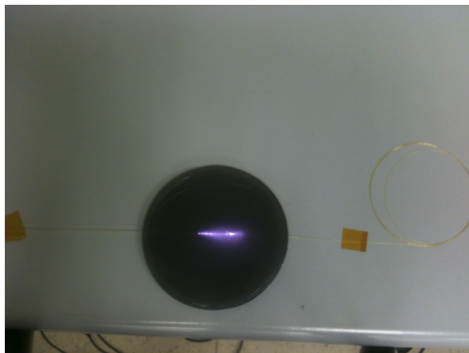
Fig. 7. The liver phantom during the thermal test. The fiber for the laser delivery is on the left side of the phantom and the fiber connected to the FBG probe is routed from the right side. Part of the laser beam is scattered outside the phantom and is detected by the camera.
