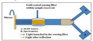
Fig. 2. Reflection based optical fiber SPR sensor set-up.
