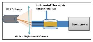
Fig. 1. Transmission based optical fiber SPR sensor set-up with intentional vertical misalignment.
