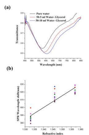
Fig. 5. (a) Transmittance of the reflection-based setup for different refractive indexes and (b) SPR wavelength shift vs refractive index for the reflection-based setup, for different repeated cycles (symbols) and linear fit (solid line).
