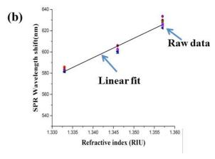
Fig. 3. Characterization of the transmission based setup: (a) example of the spectral transmittance versus wavelength for three cases; (b) notch wavelength position versus refractive index for different cycles of the experiment (symbols) and linear fit (solid line).
