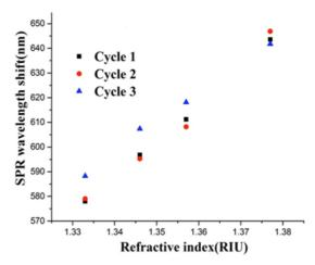
Fig. 7. Wavelength shift versus refractive index for repeated connections of the fiber probe in the reflection-based setup. The fiber is disconnected/reconnected at each cycle.
