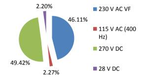
The high power share of the 270 VDC electric line has been chosen due to the low weight, high efficiency and reliability of ATRU (Auto-Transformer Rectifier Unit), also used on the Boeing 787 Dreamliner.
