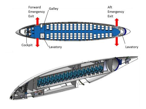
Figure 1: Internal configuration.
