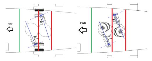
Figure 4: Main landing gear retraction angles.
