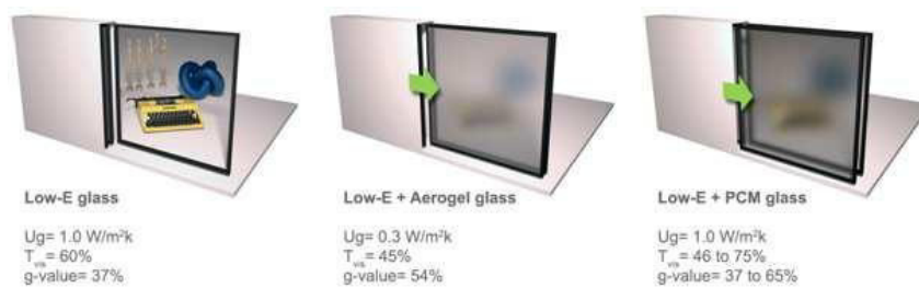
Fig. 1. Visualization of the concept of the RBE, with the two active layers sliding in front or back a static Low-E selective glazing.
