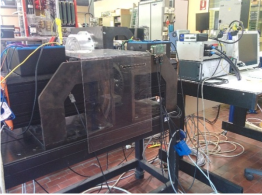
Figure 13. Experimental setup: two identical Thor motors are connected back-to-back and mounted on C-frames. On the right-hand side are the current and temperature transducers and data logger.
