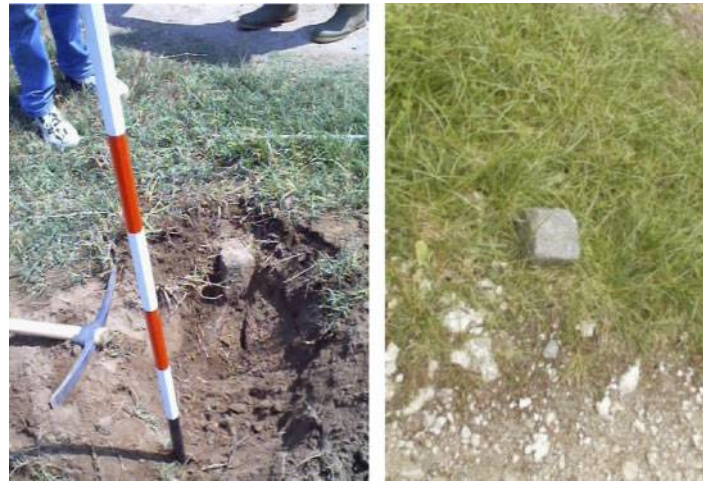
2 Boundary stone marker buried, found with GNSS measurements; boundary stone found on the ground
