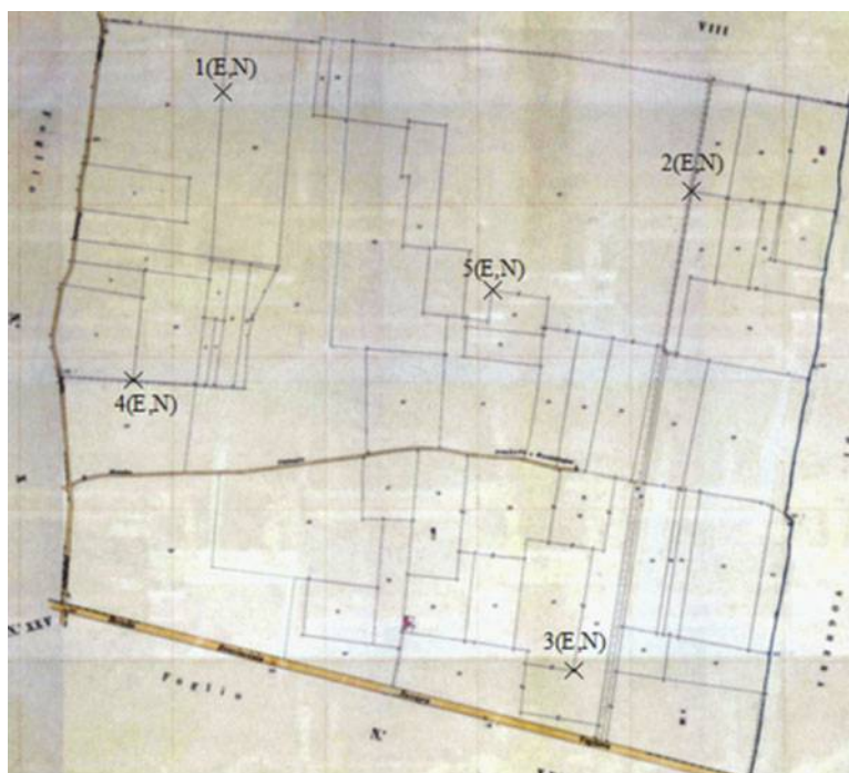
9 Location of the five points of which he wants to know the accuracy. Original scale map 1:2000
