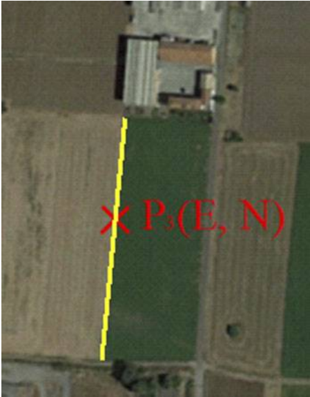
4 Condition of belonging. Measurement of the coordinates on the map (yellow line) and in the field (point P 3 )
