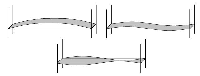
Figure 5. Some possible oscillations of a bridge roadway.
